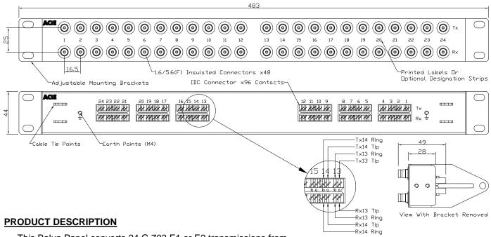
This Balun Panel converts 24 G.703 E1 or E2 transmissions from unbalanced 75 coaxial to balanced 120 twisted pair. A bi-directional device requiring no external power, it connects telecommunications equipment with mismatched interfaces or facilitates the conversion from coaxial to twisted pair distribution wiring. In addition this product offers the following features:-
