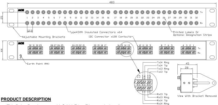
This Balun Panel converts 32 G.703 E1 or E2 transmissions from unbalanced 75 coaxial to balanced 120 twisted pair. A bi-directional device requiring no external power, it connects telecommunications equipment with mismatched interfaces or facilitates the conversion from coaxial to twisted pair distribution wiring. In addition this product offers the following features:-
